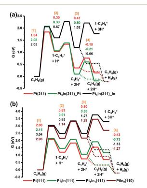
Fig. 5 (a) Gibbs free energy diagram of  $\alpha$ -type ( $C_3H_8 \rightarrow 1$ - $C_3H_7^* \rightarrow C_3H_6^* \rightarrow 1$ - $C_3H_5^*$ ) PDH reaction on Pt(211), Pt<sub>3</sub>In(211)\_Pt and Pt<sub>3</sub>In(211)\_In. (b) Gibbs free energy diagram of  $\alpha$ -type PDH reaction on Pt(111), Pt<sub>3</sub>In(111), Pt<sub>1</sub>In<sub>1</sub>(111) and PtIn<sub>2</sub>(110).
