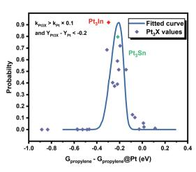
Fig. 3 The probability that the activity and selectivity of a given catalyst are better than pure Pt under given activity and selectivity constraint conditions as a function of propylene adsorption energy relative to that of Pt (Y: the difference between propylene desorption free energy barrier and further dehydrogenation step free energy barrier of Pt<sub>3</sub>X,  $k_{\text{Pt-X}}$ : the rate constants of Pt<sub>3</sub>X).
