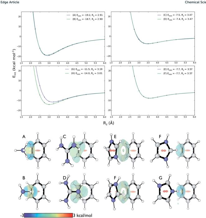
Fig. 4 Top: DLPNO-CCSD(T)/aug-cc-pVTZ interaction energies (kcal mol<sup>-1</sup>) as a function of intermolecular separation of cation $-\pi$  complexes. Minimum energies  $(E_{min})$  and equilibrium separations  $(R_r)$  shown. Bottom: NCI isosurfaces at the minimum energy separations.
