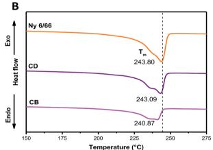
Fig. 6 DSC curves of the nylon 6/66 and CSH-nylon 6/66 nanocomposites during the first cooling (A) and second heating (B) scans.
