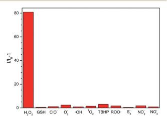
Fig. 2 FL response of the ABD system (10 μM) to a series of ROS (100 μM) in PBS buffer solution.  $I_0$  and I are the FL intensity of the ABD-system in PBS buffer solution in the presence of ROS, RNS, and RSS including  $H_2O_2$ ,  $O_2^-$ , GSH, ClO $^-$ , OH,  $^1O_2$ , TBHP, ROO $^-$ ,  $S_2^-$ , NO $_2^-$  and NO $_3^-$ . PBS buffer solution (pH = 7.8, 10 mM, containing 1% DMSO); temperature: 37 °C; excitation wavelength: 330 nm; reaction time: 100 min.
