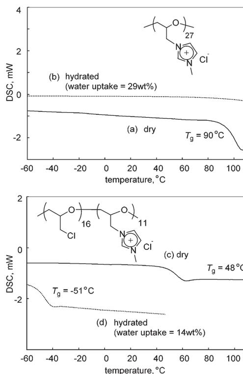
**Fig. 6** DSC thermograms (heating steps) of (a) poly(ECH-MeIm<sup>+</sup>Cl<sup>-</sup>), (b) the hydrated poly(ECH-MeIm<sup>+</sup>Cl<sup>-</sup>) (after being exposed to air (23 °C, and 40% RH) for 30 min), (c) poly(ECH-MeIm<sup>+</sup>Cl<sup>-</sup><sub>40%</sub>) and (d) the hydrated poly(ECH-MeIm<sup>+</sup>Cl<sup>-</sup><sub>40%</sub>) after being exposed to air (23 °C, and 40% RH) for 30 min (determined under N<sub>2</sub>, at 10 °C min<sup>-1</sup> for each step).
