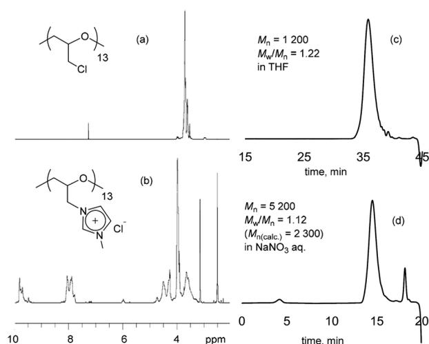
Fig. 1 <sup>1</sup>H NMR spectra of (a) poly(ECH) (in CDCl<sub>3</sub>;  $M_n = 1200$ ; DP = 13, as described in Table S1, run 5†) and (b) poly(ECH-MeIm<sup>+</sup>Cl<sup>-</sup>) (in DMSO-*d*<sub>6</sub>;  $M_{n(\text{calc})} = 2300$ ; DP = 13), and GPC chromatograms of (c) poly(ECH) and (d) poly(ECH-MeIm<sup>+</sup>Cl<sup>-</sup>).
