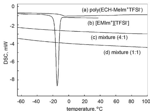
**Fig. 8** DSC thermograms (heating steps) of (a) poly(ECH-Melm $^+\text{TFSI}^-$ ) ( $M_{n(\text{calc})} = 45\,400$ , and DP = 108), (b) [EMIm $^+$ ][TFSI $^-$ ], (c) a mixture of 80 wt% [EMIm $^+$ ][TFSI $^-$ ] and 20 wt% of the poly(ECH-Melm $^+\text{TFSI}^-$ ), and (d) a mixture of 50 wt% [EMIm $^+$ ][TFSI $^-$ ] and 50 wt% of the poly(ECH-Melm $^+\text{TFSI}^-$ ) (determined under  $\text{N}_2$ , at 5 °C  $\text{min}^{-1}$  for each step).
