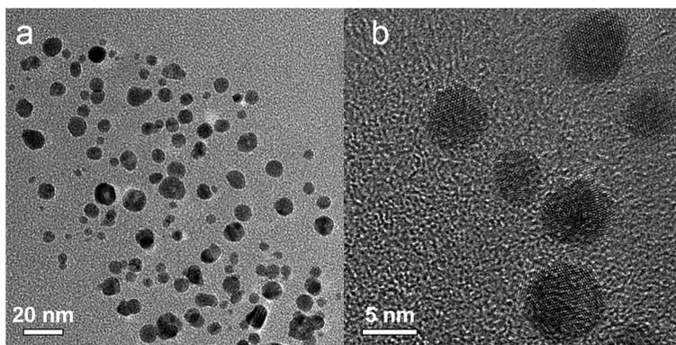
Fig. 10 (a) TEM and (b) HRTEM images of nanoparticles synthesised using only Pd(NO<sub>3</sub>)<sub>2</sub> in Reactor 3 and HQ in Reactor 4.
