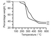
Fig. 2 TGA of 4 & 3 shown as (a) & (b) respectively.
