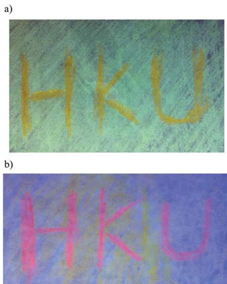
Fig. 8 An image of the weighing paper impregnated with (a) 5 and (b) 7 under UV irradiation, where "HKU" was written with a glass rod.
