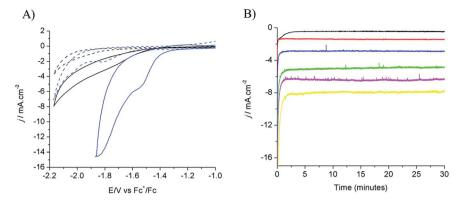
Fig. 1 (A) Cyclic voltammograms recorded on a modified Cu electrode (80 s electrodeposition) (blue) and Cu plate electrode (black) in  $[EMIM](BF_4)/H_2O$  (92/8 v/v) after  $N_2$  purging (dashed lines) and  $CO_2$  purging (solid lines). (B) Current densities during electrolysis in  $CO_2$ -saturated  $[EMIM](BF_4)/H_2O$  (92/8 v/v) at different potentials: -1.25 V (black), -1.35 V (red), -1.45 V (blue), -1.55 V (green), -1.65 V (magenta), and -1.75 V (yellow) vs.  $Fc^+/Fc$ .
