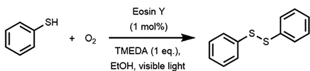
Scheme 1 Dimerization of thiophenol to diphenyl disulfide via photocatalytic aerobic oxidation with Eosin Y as photocatalyst.
