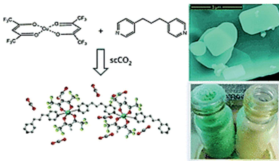
Fig. 21 The preparation of Cu(II) 1D MOFs using an eco-efficient method based exclusively on supercritical CO 2 as a solvent. [Reproduced from ref. 234 with permission from The Royal Society of Chemistry.]
