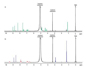
Fig. 2  $\,^{1}$ H NMR spectra of alkaline stress testing; (a) time 0, and (b) after 17 h. Signals shown in green are from voriconazole, in red from degradation product 1, and in blue from degradation product 2, both here and in subsequent figures.
