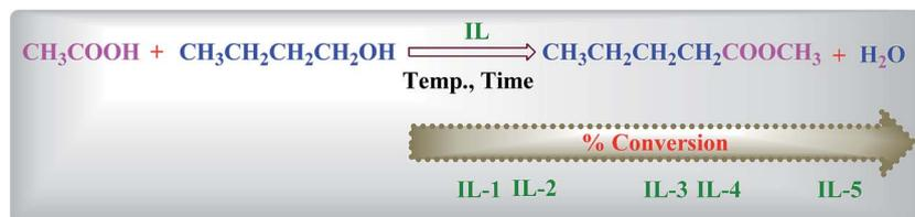
Scheme 3 Representative esterification reaction of acetic acid with *n*-butanol catalyzed by BAILs.
