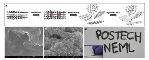
Fig. 1 (a) Schematic images depicting the procedure of fabricating conductive AqNPs/rGO hybrid powder. SEM images of (b) pure rGO and (c) synthesized AgNPs/rGO hybrid powders. (d) Letters drawn with the AgNPs/rGO pellet. Inset shows a drawing process.
