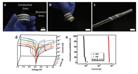
Fig. 6 Resistive switching memory devices fabricated by pencil writing. (a–c) The optical images of pencil-drawn memory devices on papers (Scale bar: 1 cm). Memory devices are fabricated on papers, so folding, bending, or wrapping can be done. (d) *I–V* characteristics of the memory device on paper. (e) Cumulative probability of high resistance state (HRS) and low resistance state (LRS) current through 38 cycles.
