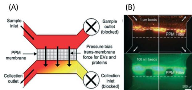
**Fig. 10** Microfluidic filtration of nanoparticles can be performed with a PPM filter with pressure-driven separation. (A) The PPM membrane passes particles smaller than the membrane pores to the collection outlet, while larger particles are retained in the sample channel. (B) shows the separation of 100 nm fluorescent beads from 1  $\mu\text{m}$  diameter beads. Reproduced from ref. 48 with permission from The Royal Society of Chemistry.
