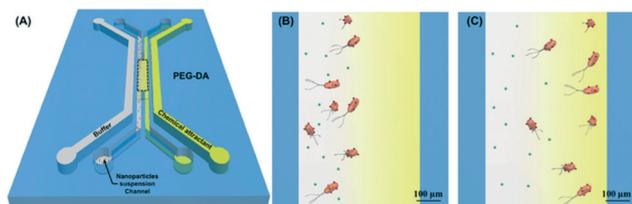
**Fig. 12** Microfluidic bacterial chemotaxis for autonomous separation of nanoparticles. (A) Channel designs for modulated diffusion of chemoattractant (B) selective attachment of nanoparticle to *E. coli* bacteria (C) chemotaxis migration of *E. coli* with attached nanoparticles. Reproduced from ref. 164 with permission from The Royal Society of Chemistry.
