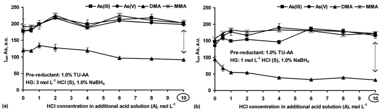
Fig. 5 Effect of the HCl concentration in the sample (S) and additional acid (A) solutions on the measurements of As(III), As(V), DMA and MMA (20 ng g<sup>-1</sup> each) by HG-ICP OES using 1.0% NaBH<sub>4</sub> and the S solutions containing 1.0% TU-AA and acidified to 3 (a) and 1 (b) mol L<sup>-1</sup> of HCl.  $I_{\text{net}}$ : the average net intensity of the As line for  $n = 3$  measurements (AA: ascorbic acid. TU: thiourea).
