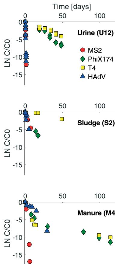
Fig. 1 Inactivation curves for MS2 (red circles),  $\Phi\text{X174}$  (green diamonds), T4 (yellow squares) and HAdV (blue triangles) in stored urine (U12), sludge (S2) and manure (M4). The complete set of inactivation curves obtained in this study are shown in the ESI† (Fig. S2 and S3).
