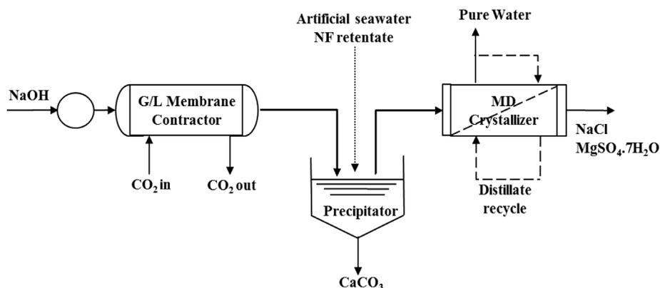
Fig. 7 Schematic flow sheet of a process of mining CaCO<sub>3</sub>, NaCl and MgSO<sub>4</sub>·7H<sub>2</sub>O from artificial seawater NF retentate using MDC (redrawn from Drioli *et al.*<sup>21</sup>).
