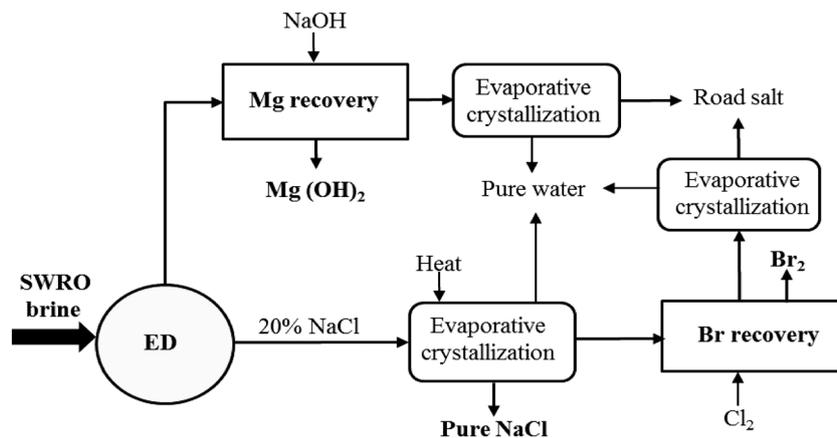
Fig. 5 Schematic illustration of SWRO brine treatment with ED and recovery of NaCl, Br<sub>2</sub> and Mg(OH)<sub>2</sub>.<sup>23</sup>
