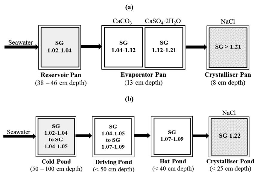
Fig. 3 Schematic illustration of salt production in (a) Goa, India<sup>56</sup> and (b) Maristella salt works at the Western Sicilian Coast.<sup>58</sup> (SG represents the specific gravity calculated from °Bé using the formula  $\text{SG} = 1.45/(1.45 - \text{°Bé})$ ).
