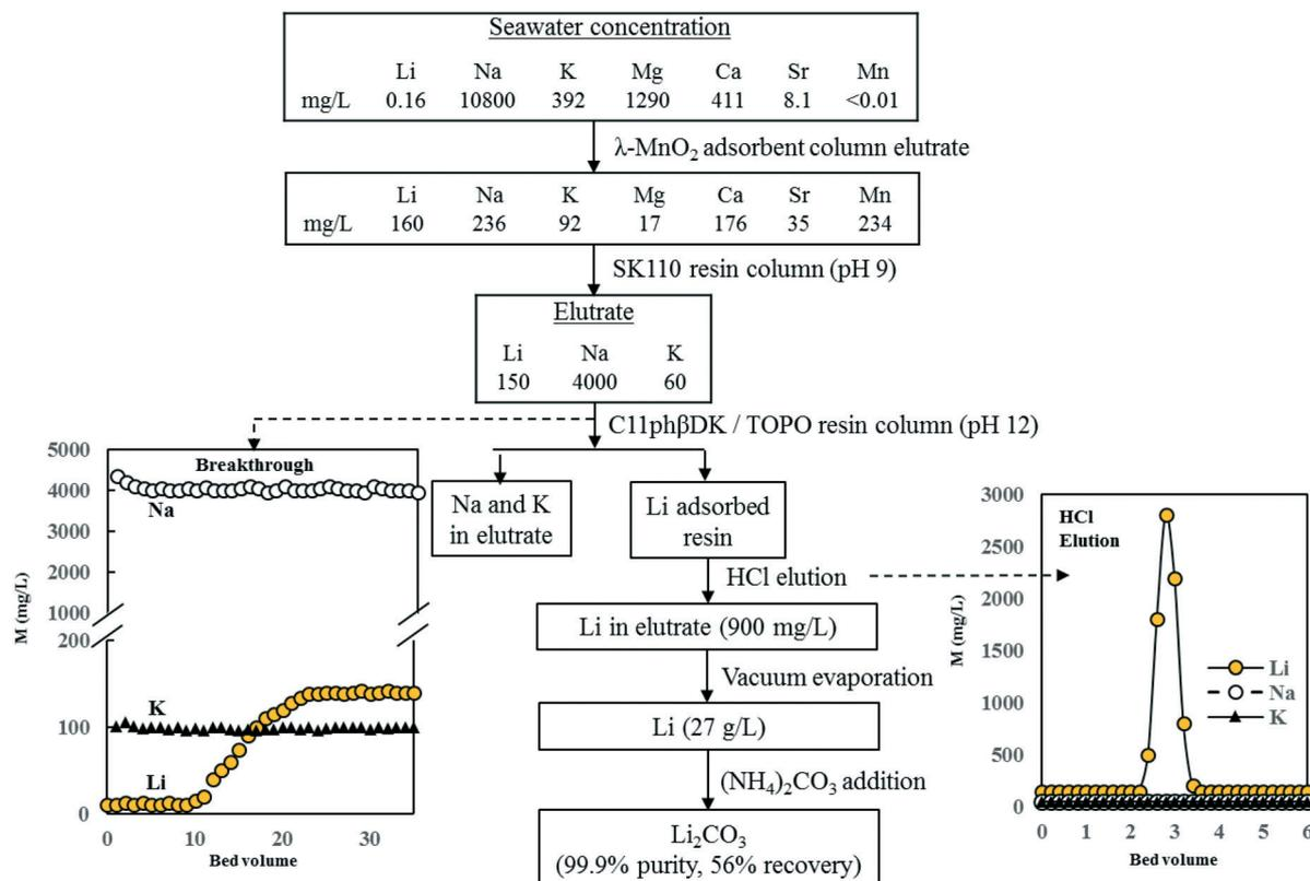
Fig. 9 Selective recovery and purification of Li from seawater (redrawn from Nishihama *et al.*).<sup>38</sup>
