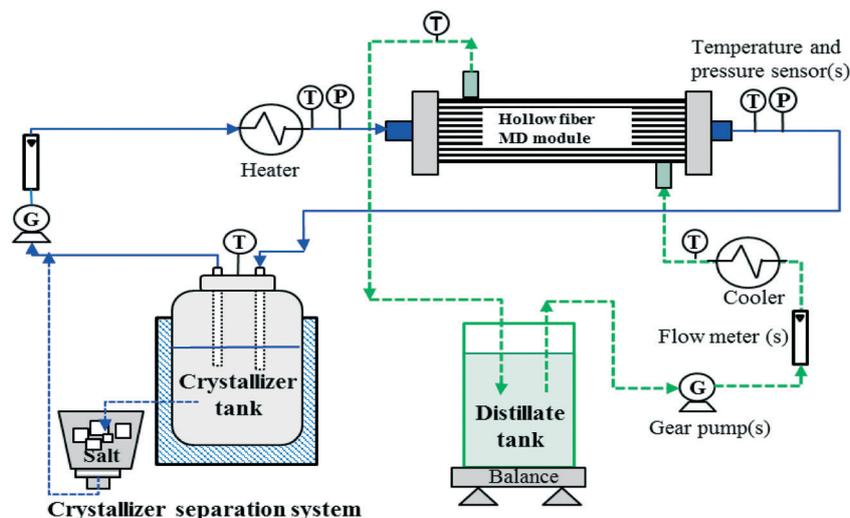
Fig. 6 Schematic flow sheet of a typical MDC (redrawn from Curcio *et al.*<sup>71</sup>).
