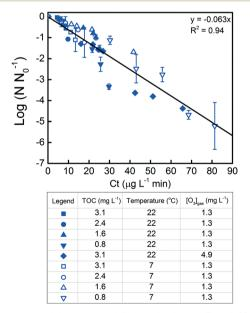
Fig. 1 Summary of L. pneumophila inactivation at 7 and 22 °C with various initial TOC loadings and initial ozone concentrations generated when the ozone generator was driven at 50 V ( $C_{gi} = 1.3 \text{ g m}^{-3}$ ) and 120 V ( $C_{qi}$  = 4.9 g m<sup>-3</sup>). Data plotted are average values and standard deviations of at least three replicates.
