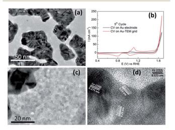
Fig. 8 HR-TEM images of (a) pristine Au grid, (b) OER performance comparison; CV were recorded at 50 mV s $^{-1}$  in 1 M NaOH, (c) Co(OH) $_2$  deposited on Au support, (d) magnified HR-TEM images showing lattice spacing of Co $_3$ O $_4$  and Au.
