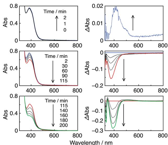
Fig. 5 UV-vis (left) and the corresponding differential absorption spectral changes (right) during the irradiation of a  $\text{CO}_2$ -saturated DMF-TEOA (5 : 1 v/v) solution containing **R(5)** (0.05 mM) as a PS and **Re-ACN** (0.05 mM) as the catalyst, under irradiation at  $\lambda_{\text{ex}} = 436$  nm ( $5.7 \times 10^{-9}$  einstein per s) in the initial stage (top) and over 3.5 h irradiation (middle and bottom).
