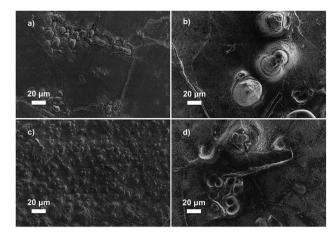
Fig. 6 Scanning electron microscopy images of a short-circuited Li anode after galvanostatic (a) polarization (0.40 mA cm $^{-2}$ ) and (c) cycling (0.26 mA cm $^{-2}$ ) test with hPNB–PEO electrolyte (plasticized with 32 wt% PEG 275) and (b) polarization (0.40 mA cm $^{-2}$ ) and (d) cycling (0.26 mA cm $^{-2}$ ) test with PCOD–PEO electrolyte (plasticized with 32 wt% PEG 275).
