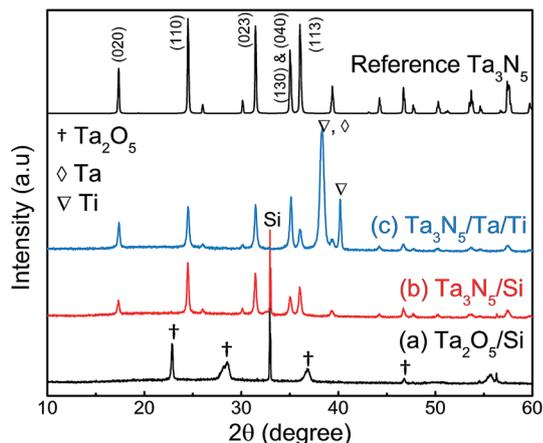
Fig. 2 XRD patterns for (a)  $\text{Ta}_2\text{O}_5/\text{Si}$  and (b)  $\text{Ta}_3\text{N}_5/\text{Si}$  obtained from the nitridation of  $\text{Ta}_2\text{O}_5/\text{Si}$ , and (c)  $\text{Ta}_3\text{N}_5/\text{Ta}/\text{Ti}$  after the transfer process. The standard pattern for the  $\text{Ta}_3\text{N}_5$  phase (PDF# 89-5200) is displayed at the top as a reference.
