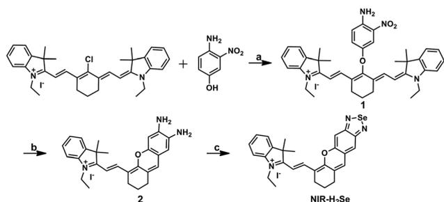
Scheme 1 Synthesis of **NIR-H<sub>2</sub>Se**. Reaction conditions: (a) NaH, DMF, rt, 73%; (b) SnCl<sub>2</sub>, HCl, CH<sub>3</sub>OH, 70 °C, 45%; (c) SeO<sub>2</sub>, grind, 71%.
