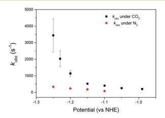
Fig. 3 Plot of  $k_{\rm obs}$  of catalyst 2, calculated from the intercepts of Koutecký–Levich plots, vs. potential at pH 2. Values are obtained averaged from 3 independent measurements with the error bars calculated from the uncertainties in the intercepts of the Koutecký–Levich plots.
