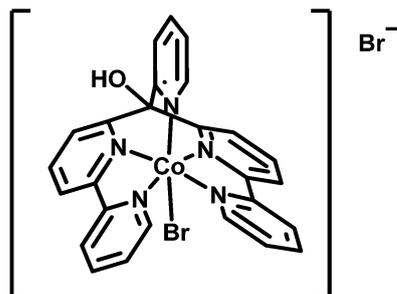
Scheme 1 Structure of water reducing catalyst  $[\text{Co}^{\text{II}}\text{Br}(\text{appy})]\text{Br}$  **1**.<sup>52,54</sup>
