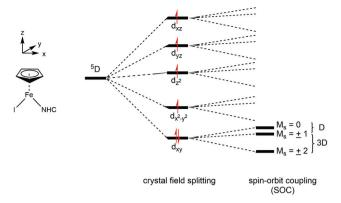
Fig. 4 Schematic illustration of the crystal field splitting and spin-orbit coupling for the <sup>5</sup>D (3d<sup>6</sup>) term.
