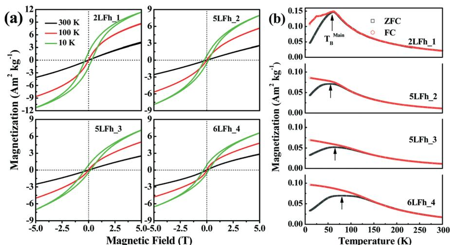
**Fig. 5** Magnetization of the four ferrihydrite samples. Panel (a) shows the hysteresis loops measured at 10, 100 and 300 K. Note that the hysteresis loops did not attain saturation at 5 T. Panel (b) shows the zero field-cooled (ZFC, black) and field-cooled (FC, red) induced magnetizations obtained with an applied field of 20 mT.
