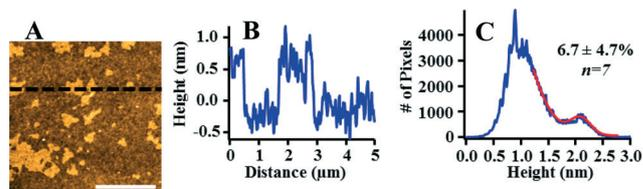
**Fig. 3** Atomic force microscopy confirms (A) the presence of distinct  $L_o$  and  $L_d$  phases with (B) the expected  $\sim 1$  nm height difference between phases in a supported lipid bilayer consisting of 60/20/20 mol% DOPC/SM/Chol. (C) The coverage of  $L_o$  domains was determined by fitting the AFM image height distribution. Scale bar is 2  $\mu\text{m}$ . AFM images of other compositions investigated are provided in Fig. S2.†
