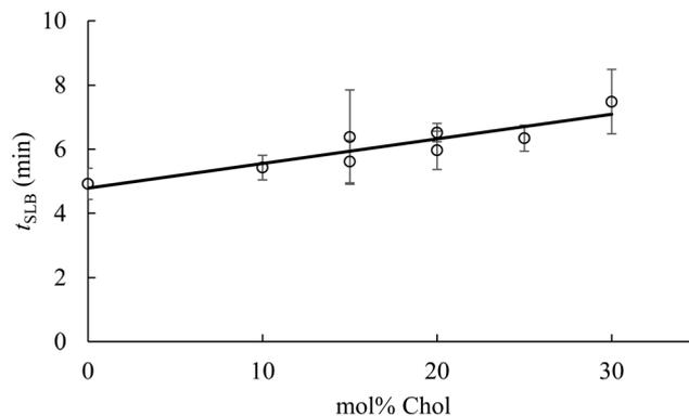
**Fig. 5** Supported lipid bilayer formation time ( $t_{\text{SLB}}$ ) as a function of vesicle cholesterol content as monitored by QCM-D. Supported lipid bilayer formation time was calculated from the time that vesicles were first observed adhering to the sensor surface to the time of initiation of vesicle rupture (as evidenced by the abrupt decrease in  $\Delta D_5$ ). Fit ( $y = 0.077x + 4.782$ ) was obtained using a standard least squares analysis ( $R^2 = 0.82$ ).
