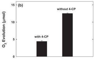
Fig. 2 (a) Time-profiled production of  $H_2$  and  $O_2$  in the suspension of  $Cr_2O_3/Rh/SrTiO_3$  and  $Rh/SrTiO_3$  with 4-CP (300  $\mu$ M) in the initially de-aerated suspension. (b) Comparison of photocatalytic  $O_2$  evolution in the suspension of  $Cr_2O_3/Rh/SrTiO_3$  (after 3 h reaction) in the presence and absence of 4-CP.
