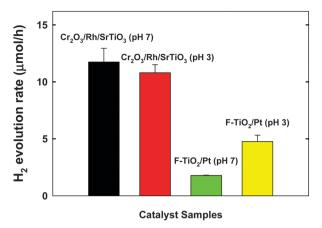
Fig. 3 Comparison of the initial photocatalytic  $H_2$  production rate between  $Cr_2O_3/Rh/SrTiO_3$  and  $F-TiO_2/Pt$  photocatalytic systems in the presence of 4-CP (300  $\mu$ M). Experimental conditions: [catalyst] = 0.5 g L<sup>-1</sup>,  $\lambda > 320$  nm, air-tight and initially Ar-purged for 1 h before UV irradiation.
