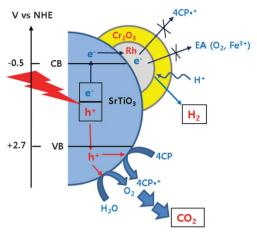
Scheme 1 Schematic illustrations of photocatalytic reaction mechanisms occurring on the surface of Cr<sub>2</sub>O<sub>3</sub>/Rh/SrTiO<sub>3</sub>.
