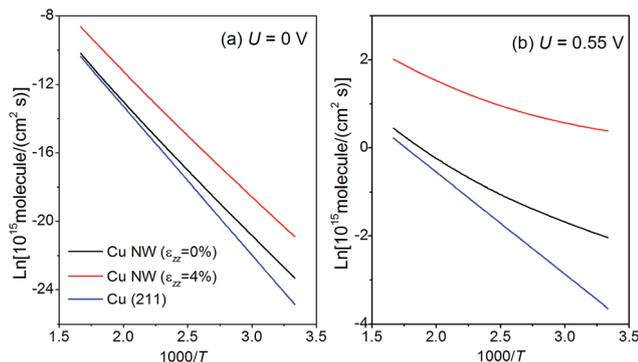
Fig. 7 Arrhenius plot for CH<sub>4</sub> production under a bias potential of (a)  $U = 0$  V and (b)  $U = 0.55$  V on both the penta-twinned Cu NW ( $d = 24$  nm) and Cu (211) surface. The temperature  $T$  varies from 300 K and 600 K.
