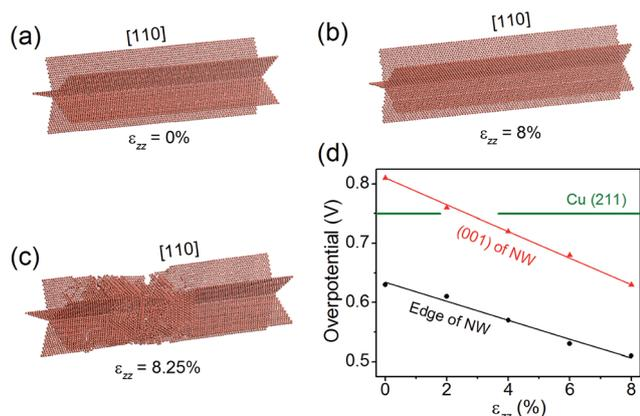
Fig. 6 (a–c) The atomic structure of the penta-twinned Cu NW under  $\epsilon_{zz} = 0\%$ ,  $8\%$  and  $8.25\%$ . Only the twin boundaries and other lattice defects are shown. (d) Overpotential on the NW edge and (001) facet as functions of uniaxial tension  $\epsilon_{zz}$ . The green horizontal line indicates the overpotential on the Cu (211) surface.
