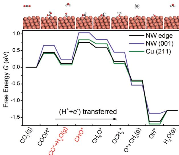
Fig. 3 The free energy diagrams of  $\text{CO}_2$  electroreduction on the NW edge, the NW (001) facet and the Cu (211) surface at 0 V vs. RHE. The two intermediates shown in red indicate the overpotential-determining step. The large orange spheres represent Cu atoms, and the small spheres represent O (red), C (gray) and H (white) atoms.
