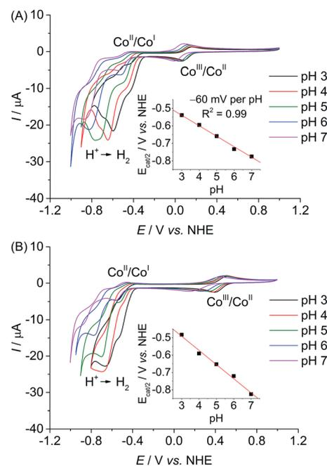
Fig. 2 CVs with dissolved (A) **CoP**<sup>3</sup> and (B) **CoP**<sup>2</sup> (0.8 mM) recorded in an aqueous Britton–Robinson buffer at different pH values on a glassy carbon working electrode at 20 mV s<sup>-1</sup>. The insets show the correlation between the half-wave potential of the catalytic reduction wave, *E*<sub>cat/2</sub>, and the pH value. The red traces represent the linear fit of the data points.
