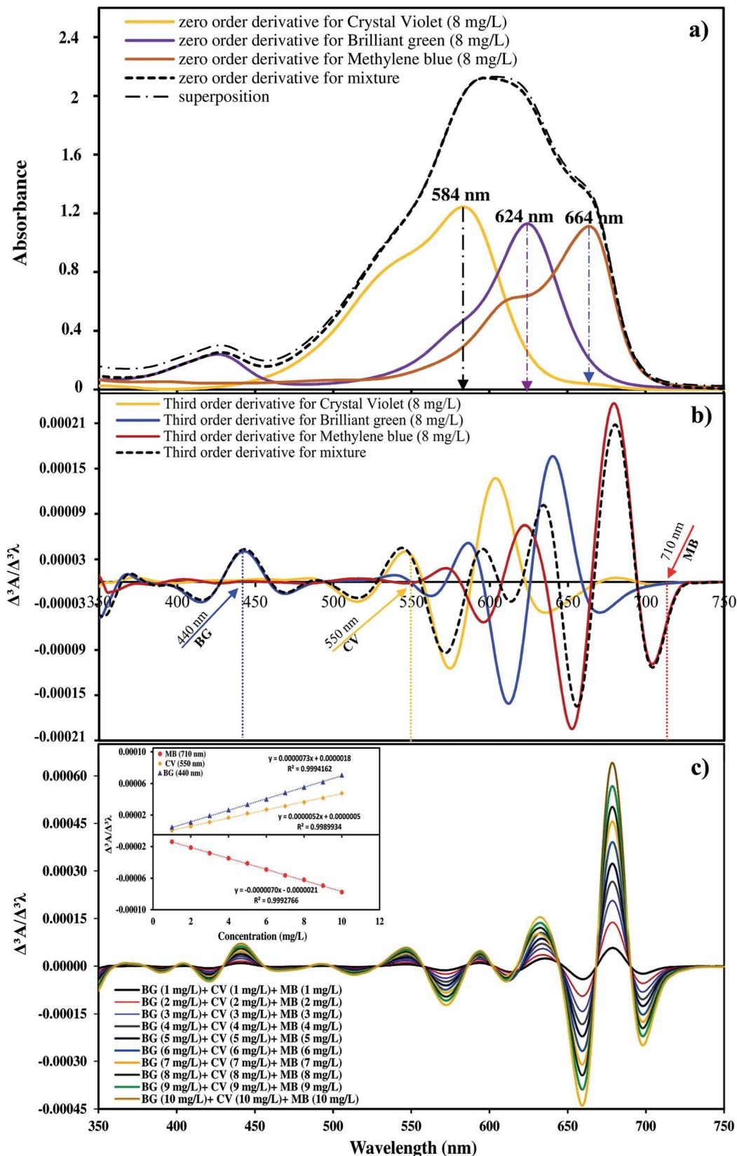
Fig. 3 (a) Zero order absorption spectra of CV, BG and MB in single and ternary solutions (with an initial dye concentration of  $8 \text{ mg L}^{-1}$  for each dye). (b) Third order derivative spectra of CV, MG and MB in ternary solutions. (c) Calibration graph at 710 nm for MB, 550 nm for CV and 440 nm for BG.
