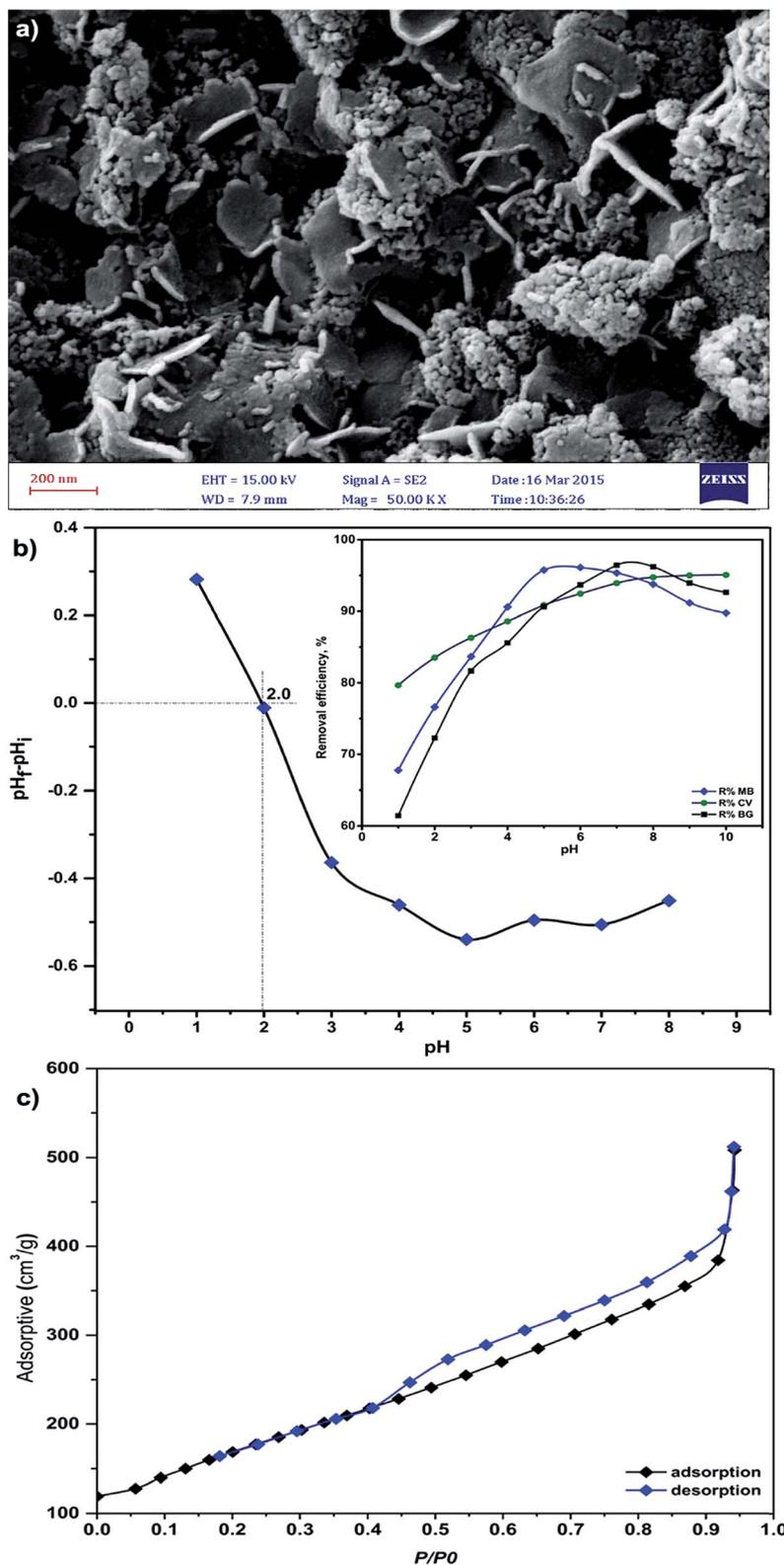
Fig. 4 (a) FESEM image of the prepared  $\text{MnO}_2$ -NP-AC, (b) pHzpc of  $\text{MnO}_2$ -NP-AC ( $\text{pH}_i$  = initial pH and  $\text{pH}_f$  = final pH) and (c) nitrogen adsorption–desorption isotherms.
