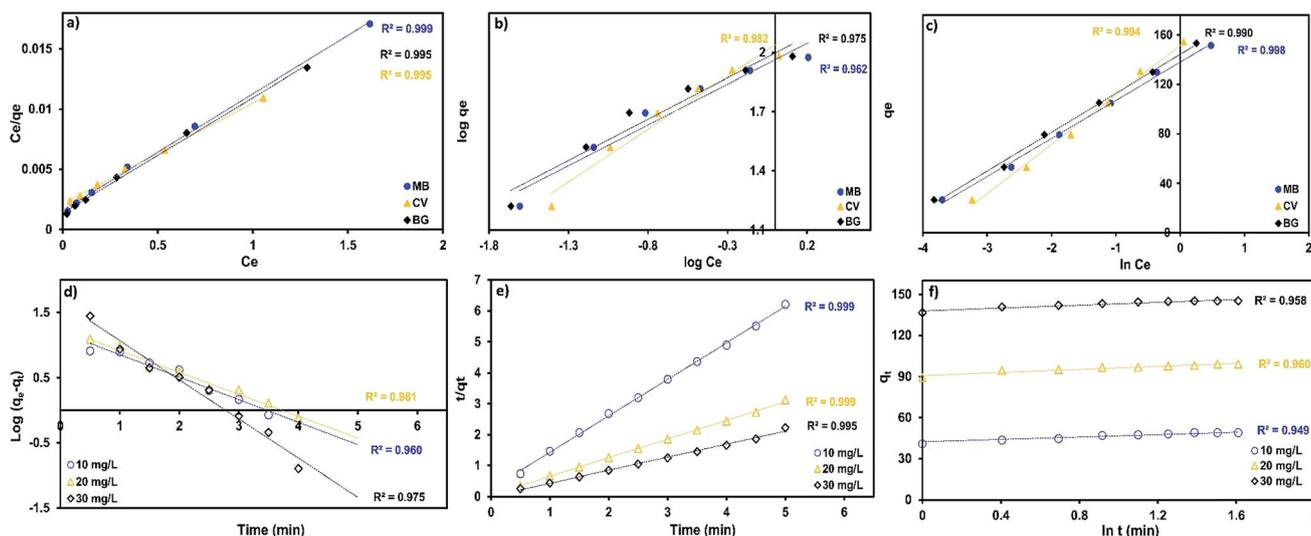
Fig. 10 Data obtained for dye adsorption on MnO<sub>2</sub>-NP-AC at different initial concentrations of dyes used to determine the isotherm parameters: (a) Langmuir, (b) Freundlich and (c) Temkin ( $C_0 = 5$ – $30$  mg L<sup>-1</sup>, adsorbent dosage = 0.01 g, sonication time = 4 min, pH = 7.0), (d) pseudo-first order, (e) pseudo-second-order kinetic and (f) Elovich plots for CV adsorption on MnO<sub>2</sub>-NP-AC.
