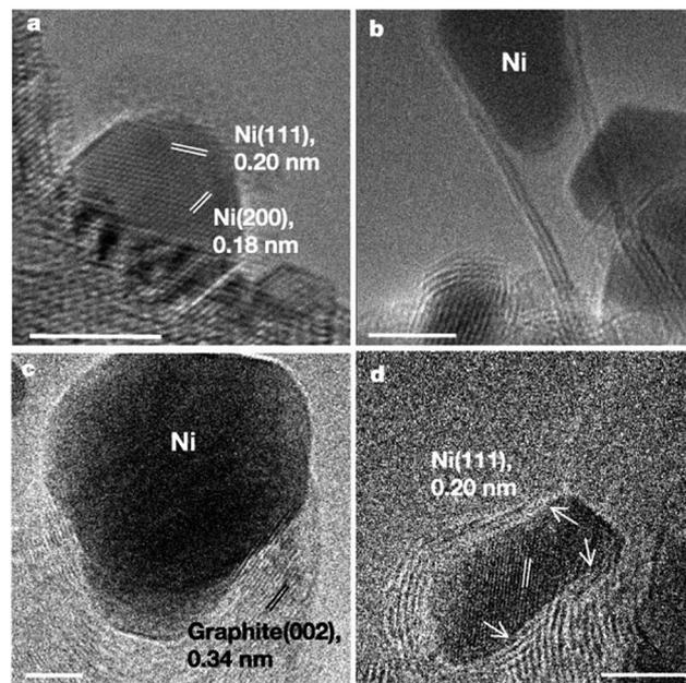
Fig. 6 Electron micrographs of the Ni catalyst and carbon nanofibres. (a) TEM image of a Ni nanocrystal supported on  $\text{MgAl}_2\text{O}_4$ . (b) TEM image showing a multi-walled tubular carbon nanofibre structure. (c) *In situ* TEM image showing a whisker-type carbon nanofibre. (d) *In situ* TEM image showing a Ni nanocrystal during carbon nanofibre growth. Scale bars, 5 nm. Reprinted by permission from Macmillan Publishers Ltd: [Nature] (ref. 84), Copyright (2004).
