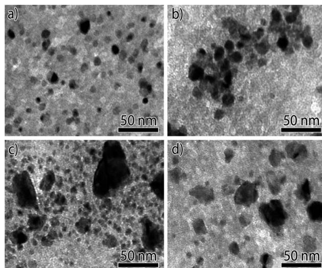
Fig. 8 TEM images of Ni/SiO<sub>2</sub> catalysts with different Ni particle sizes after 150 h on-stream (230 °C, H<sub>2</sub> : CO = 2 : 1, 0.1 MPa). (a) ~8 nm, (b) ~9 nm, (c) ~4 nm, and (d) ~3 nm. Reproduced with permission from ref. 66 Copyright (c) [2014 WILEY-VCH Verlag GmbH & Co. KGaA, Weinheim].
