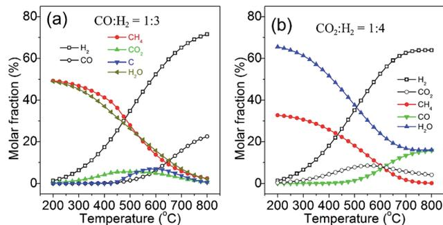
Fig. 2 Product compositions for CO (a) and CO<sub>2</sub> (b) methanation at equilibrium (0.1 MPa). Adapted from ref. 24 with permission of the Royal Society of Chemistry.
