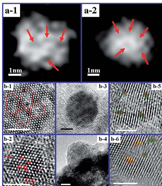
Fig. 5 (a-1 and a-2) High-angle annular dark field (HAADF) STEM images of Ni nanoparticles in Ni/H- $\text{Al}_2\text{O}_3$ . (b-1–b-6) HRTEM images of Ni nanoparticles selected from the Ni/H- $\text{Al}_2\text{O}_3$  sample (the scale bar is 2 nm). Reprinted with permission from ref. 52 Copyright (2013) American Chemical Society.
