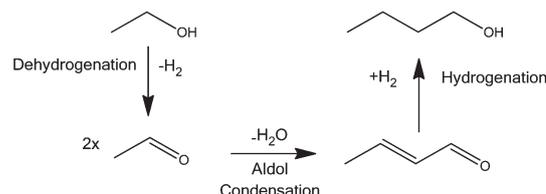
**Scheme 1** The Guerbet reaction: dehydrogenation of EtOH to acetaldehyde, followed by aldol condensation of acetaldehyde to form crotonaldehyde; finally BuOH is formed *via* hydrogenation of crotonaldehyde.
