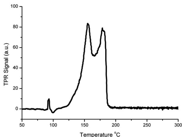
**Fig. 2** Results of temperature programmed reduction of the unreduced Cu/HSACeO<sub>2</sub> catalyst immediately following calcination; two well separated peaks can be seen at 155 and 178 °C, these two peaks are tentatively assigned to non-crystalline CuO interacting with CeO<sub>2</sub> and larger non-crystalline CuO associated with CeO<sub>2</sub> respectively.
