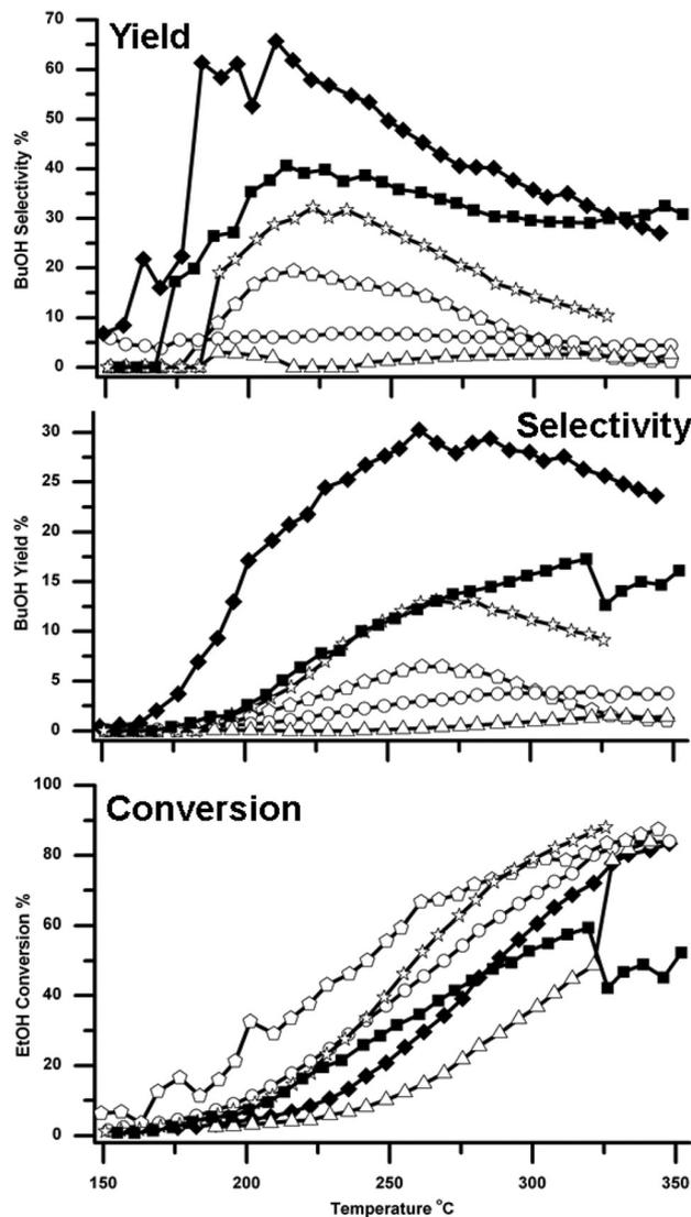
Fig. 3 Traces showing how the yield of BuOH, selectivity to BuOH and conversion of EtOH, vary over the six different catalysts. The traces are marked as follows  $\circ$  Cu/Al<sub>2</sub>O<sub>3</sub>,  $\triangle$  Cu/ZSM-5 SAR-80,  $\star$  Cu/TiO<sub>2</sub>,  $\diamond$  Cu/Si/Al,  $\blacksquare$  Cu/CeO<sub>2</sub> and  $\blacklozenge$  Cu/HSA CeO<sub>2</sub>. Note that, although the yields varied, some BuOH was formed over all six catalysts.
