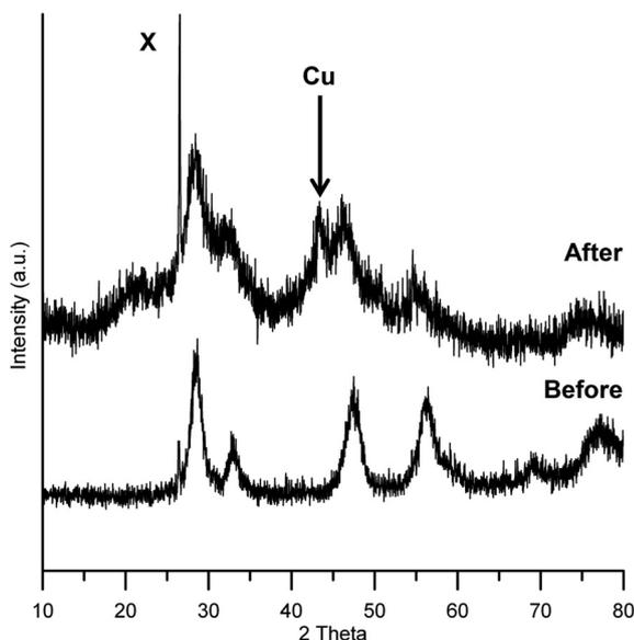
**Fig. 1** pXRD pattern of Cu/HSACeO<sub>2</sub> catalyst before and after reaction. Only one peak can be tentatively assigned to a Cu or CuO phase either before or after reduction. The pattern for the catalyst after reaction indicates a more amorphous structure possibly due to the formation of Ce<sub>2</sub>O<sub>3</sub> phases [The sharp peak at 26 2θ° X is from the brass insert used in the sample holder].
