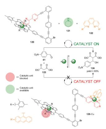
Scheme 33 Switchable catalysis of a Knoevenagel reaction based on the capture/release of a piperidine catalyst (121) by Zn(III)-porphyrin 120 induced by the reversible coordination of Cu(II).
