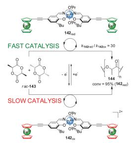
Scheme 39 Influencing the rate of polymerization of rac-lactide (143) by oxidation/reduction of ferrocene groups pendant to a Ti(IV)-salen catalyst (142).<sup>71</sup>
