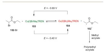
Scheme 43 Electrochemical control over the activation of a polymerization reaction by reduction/oxidation of Cu(ı)/Cu(ıı).76
