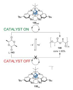
Scheme 44 'On-off' switching of lactide polymerization catalyst 155 triggered by reduction/oxidation of the cerium catalytic centre. 77
