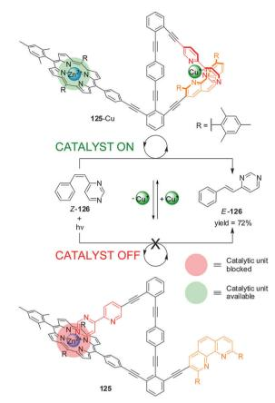
Scheme 34 Control of the activity of catalyst **125** in a *cis-trans* isomerization process triggered by the addition/removal of Cu(ı).<sup>65</sup>
