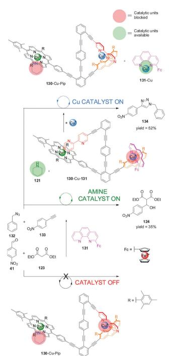
**Scheme 36** Switching of catalytic system **130** between an 'off' state and two 'on' states with orthogonal catalytic processes through the sequential addition of phenanthroline derivative **131** and Cu(i).<sup>67</sup>
