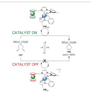
Scheme 41 Control over the activity of metathesis catalyst 146 by change of the oxidation state of a ferrocene iron centre.<sup>73</sup>
