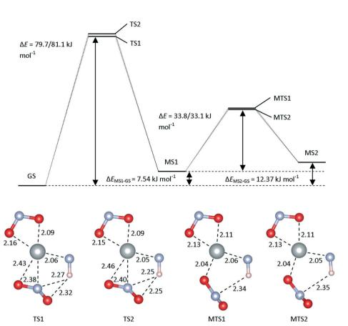
Fig. 4 Schematic of the isomerisation pathways in  $[Ni(Et_d dien)(\eta^2 - O,ON)(\eta^1 - NO_2)]$ , modelled using the M06 functional and the LANL2DZ/6-311++G(d,p) basis set, and with water as a continuum. The energy profile illustrates the relative energies of the GS, MS1 and MS2 isomers, and the transition states connecting them, while the four models show the optimised geometries of the four transition states.
