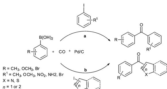
**Scheme 45** Reagents and conditions: (a) aryl iodide (1 mmol), arylboronic acid (1.2 mmol),  $CO$  (200 psi), 10%  $Pd/C$  (2 mol%),  $K_2CO_3$  (3 mmol), anisole (10 mL),  $100^\circ C$ , 8 h; (b) heteroaryl iodide (1 mmol), arylboronic acid (1.2 mmol),  $CO$  (200 psi), 10%  $Pd/C$  (2.5 mol%),  $K_2CO_3$  (3 mmol), toluene (10 mL), time 10 h, temp.  $100^\circ C$ .
