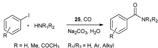
**Scheme 31** Reagents and conditions: aryl iodide (1 mmol), amine (2 mmol), Na<sub>2</sub>CO<sub>3</sub> (2 mmol), **25** (50 mg, 14.2 μmol), water (10 mL), CO pressure (100 psi), temp. 100 °C, time 8 h.
