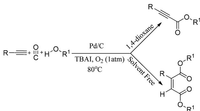
**Scheme 43** Reagents and conditions: alk-1-yne (1 mmol), alcohol (0.5 mL), 10% Pd/C (10 mol%),  $CO/O_2$  (5 : 1 atm), TBAI (0.6 mmol), 1,4-dioxane (10 mL), temp.  $80^\circ C$ , time 8 h. (The unsymmetrical maleate esters were formed directly by using the alcohol as the solvent under the same reaction conditions).
