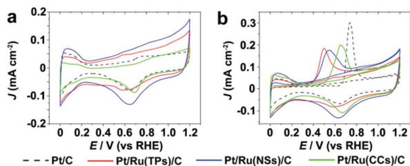
Fig. 7 (a) CV curves of Pt/C and Pt/Ru NCs/C composites in 0.1 M HClO<sub>4</sub> at the scanning rate of 50 mV s<sup>-1</sup>. (b) The first cycle and the forward scan of the second cycle of CO stripping tests in 0.1 M HClO<sub>4</sub> at the scanning rate of 50 mV s<sup>-1</sup>.
