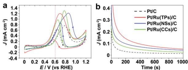
**Fig. 5** (a) Stable CV curves of Pt/C and Pt/Ru NCs/C composites in 0.1 M HClO<sub>4</sub> and 0.1 M MeOH at the scanning rate of 50 mV s<sup>-1</sup>. A violet dashed vertical line marks 0.6 V vs. RHE. (b) *i*–*t* curves in 0.1 M HClO<sub>4</sub> and 0.1 M MeOH at 0.6 V vs. RHE. The current density of different catalysts was normalized in reference to the ECSA obtained from CO stripping tests.
