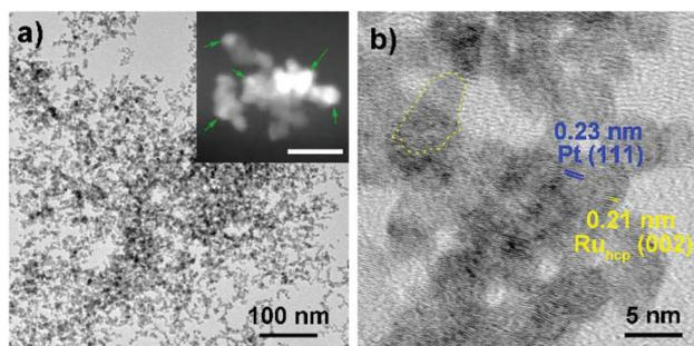
**Fig. 3** TEM characterization of Pt/Ru NSs nanocomposites. (a) shows the TEM image and the inset shows HAADF-STEM image (scale bar: 20 nm). Pt particles are marked by green arrows. (b) shows the HRTEM image. A poorly crystallized region is enclosed by a cycle of yellow dashed line.
