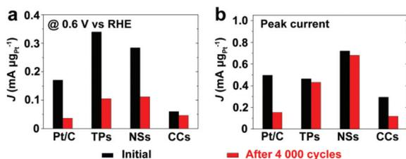
**Fig. 9** Mass specific activity (a) at 0.6 V vs. RHE and (b) at peak current of forward scan of different catalysts before and after 4000 cycles of voltage scan. TPs, NSs and CCs in this figure stand for Pt/Ru TPs/C, Pt/Ru NSs/C and Pt/Ru CCs/C, respectively.
