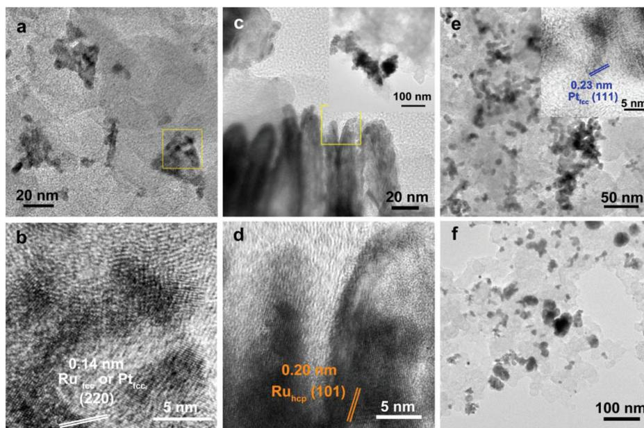
**Fig. 8** TEM and HRTEM images of (a and b) Pt/Ru TPs/C, (c and d) Pt/Ru CCs/C, (e) Pt/Ru NSs/C and (f) commercial Pt/C after 4000 cycles of voltage scan in HClO<sub>4</sub>-MeOH mixed solution. Inset of c shows a low-magnification TEM image of Pt/Ru CCs/C and inset of e shows a HRTEM image of Pt/Ru NSs/C. HRTEM images b and d were taken from the regions marked with yellow frames in a and c, respectively.
