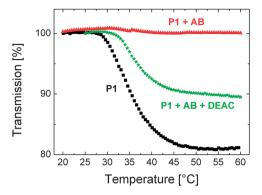
Fig. 7 Temperature-transmission profile of the aqueous solution of P1 (0.01 g  $L^{-1}$ , black squares), containing 0.17  $\mu$ M of antibody (red triangles), and containing both the antibody (0.17 µM) and the DEAC-labelled monomer (4 µM) (green stars). The profiles were recorded for the same solutions labelled a, b, and d of Fig. 6.
