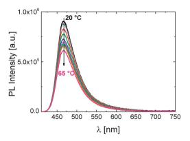
**Fig. 8** The effect of temperature on the fluorescence characteristics of **P2** in PBS  $(0.15 \text{ g L}^{-1})$ . The excitation wavelength is 400 nm. The direction of the arrow shows the increase in the solution temperature from 20 to 65 °C.
