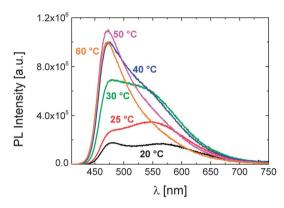
Fig. 2 The evolution of the PL spectra of P1 in PBS (0.15 g  $L^{-1}$ ) with temperature, recorded at an excitation wavelength of 400 nm.
