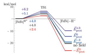
**Fig. 3** Energy profiles for the reaction [FeFe] $^{H+} \rightarrow TS1 \rightarrow [FeFe] - H^-$  for different field strengths. The barriers are given in kcal mol<sup>-1</sup>.
