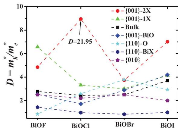
**Fig. 4** Variation of  $D$  with BiOX structures. For clarity and harmony, the relative ratio  $D$  of the 2-layer Cl terminated BiOCl {001} facet, which has a numerical value of 21.95, is shown as 9 in this figure. Dashed lines are guides for eyes.
