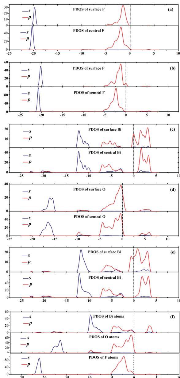
**Fig. 5** Partial density of states (PDOS) for surface and central (a) F atoms within {001}-1F, (b) F atoms within {001}-2F, (c) Bi atoms within {001}-BiO, (d) O atoms within {110}-O, and (e) Bi atoms within {110}-BiF. (f) is the PDOS of the BiOF with {010} surface. Dashed lines represent the Fermi level at 0 eV.
