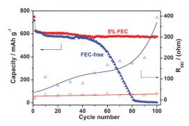
Fig. 3 Changes of the cycling capacities and SEI film resistances of the Sb/C anodes in the 1.0 mol  $L^{-1}$  NaPF<sub>6</sub> + EC-DEC electrolyte with (red  $\blacksquare \Box$ ) and without (blue  $\blacktriangle \triangle$ ) the addition of 5% FEC additive.
