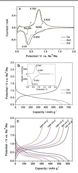
Fig. 2 Electrochemical properties of the Sb/C nanocomposite: (a) The CV curve at a scan rate of 0.1 mV s<sup>-1</sup> (vs. Na<sup>+</sup>/Na); (b) charge-discharge curves of the Sb/C composite at a constant current of 100 mA g<sup>-1</sup>, the inset is differential capacity versus cell potential curve; (c) charge-discharge profiles at various current densities from 150 mA  $g^{-1}$  to 2000 mA  $g^{-1}$ .
