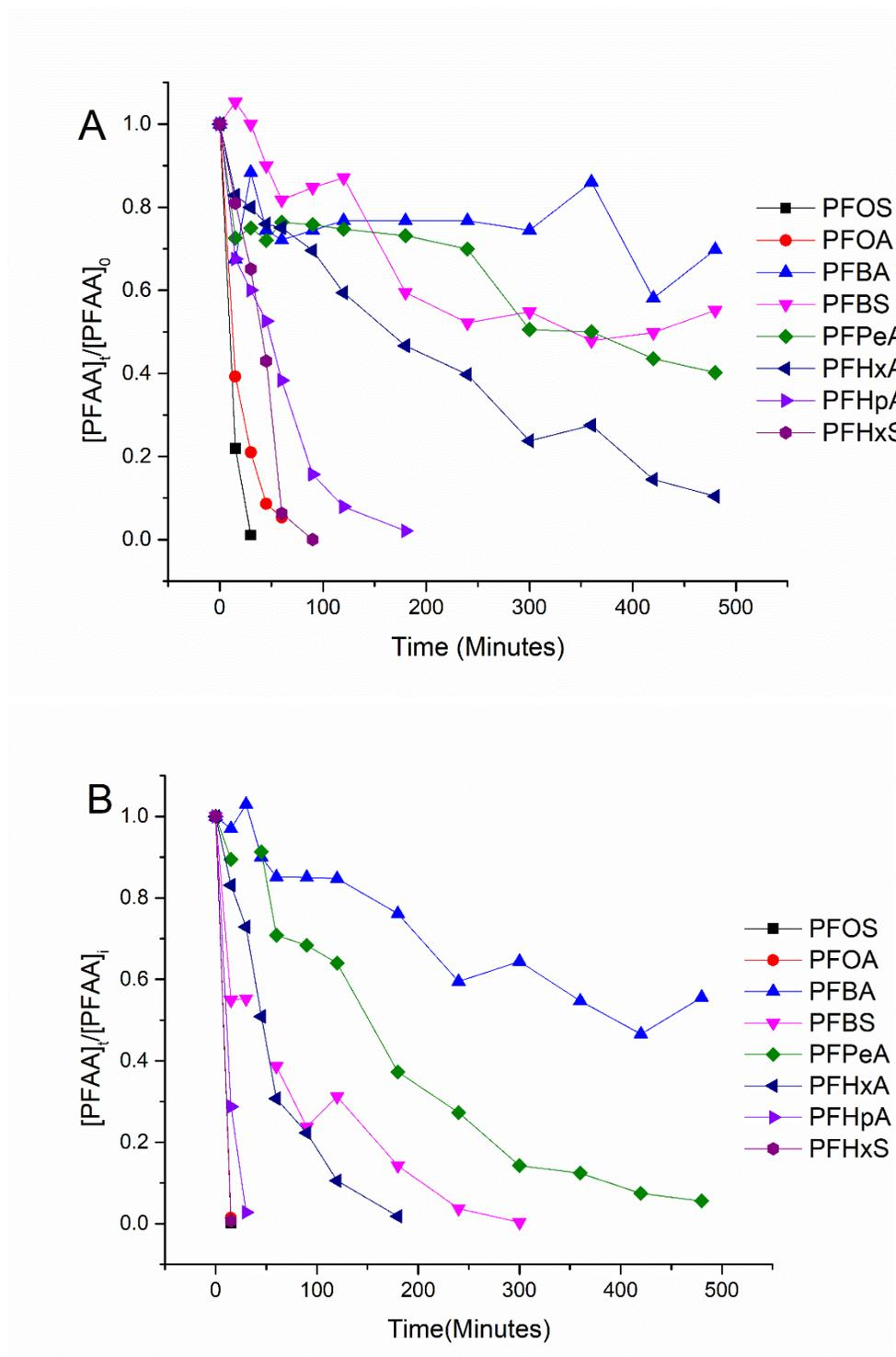
**Figure 2.** The concentration of each PFAA over time during electrooxidation with TSO anode at 5 mA·cm<sup>-2</sup> (A) and 15 mA·cm<sup>-2</sup> (B). The test solutions contained all PFAAs in mixture with each at the initial solution of was 2.0  $\mu$ M in 100-mM Na<sub>2</sub>SO<sub>4</sub> as supporting electrolyte.
