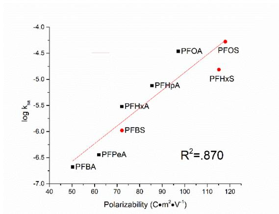
Effective degradation of eight perfluoroalkyl acids by electrooxidation on titanium suboxide anode is correlated to their respective molecular structures, offering insight into their degradation behaviors.
