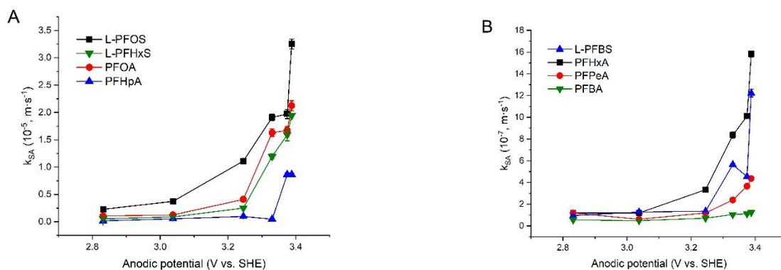
**Figure 4.** The  $k_{SA}$  values of 8 PFAAs plotted against the anodic potential vs. SHE (standard hydrogen electrode) for electrooxidation. The test solutions contained all PFAAs in mixture with each at the initial solution of was  $2.0 \mu\text{M}$  in  $100\text{-mM Na}_2\text{SO}_4$  as supporting electrolyte. Error bar represents standard deviation. The data are shown in two figures according to magnitudes for better observation.
