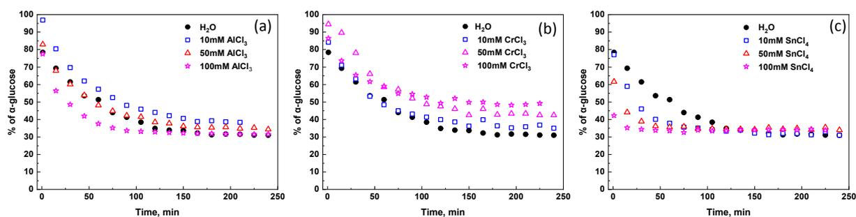
Figure 3: Kinetics profiles from in-situ Raman spectroscopic data. Analysis has been performed by utilizing the  $I_{543}/(I_{543} + I_{448})$  ratio of skeletal modes of glucose
