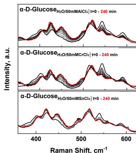
Figure 1: In situ Raman spectra of glucose mutarotation reaction
