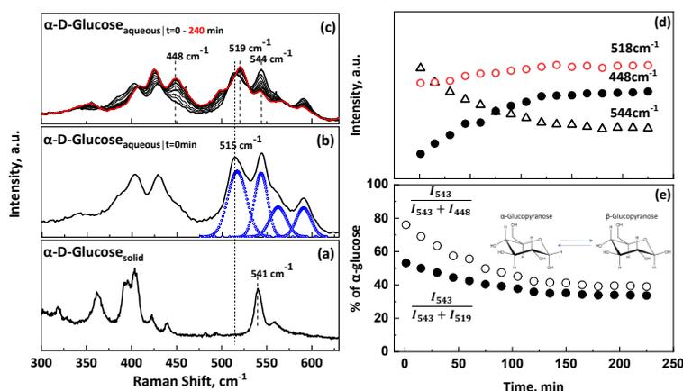
Figure 1: Raman spectrum of  $\alpha$ -glucose in a) solid, b) water and c) under mutarotation reaction. Analysis of spectra is shown in d) and e).
