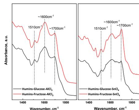
Figure 4: ATR-FTIR spectra of humins formed in  $\text{AlCl}_3$  and  $\text{SnCl}_4$  solutions
