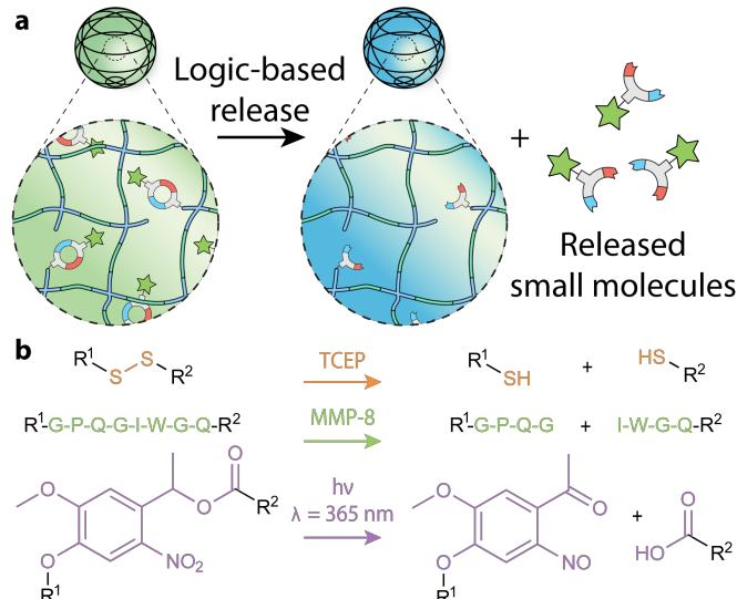
**Fig. 1** (a) Small molecules conjugated to hydrogel biomaterials through degradable linkages of defined molecular architecture undergo triggered release in response to precise combinations of environmental inputs following Boolean logic. (b) Disulfide-,  $-GPQGIWGQ-$  peptide-, and *ortho*-nitrobenzyl ester-containing linkers are cleaved in response to TCEP, MMP-8, and light, respectively.
