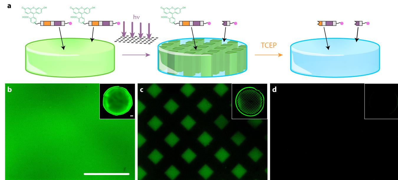
**Fig. 5** (a) Gels containing FAM-RVP exhibit sequentially triggered release in response to masked light followed by reductive treatment. Fluorescent images of gels (b) prior to treatment (<sub>N</sub>), after (c) exposure to photomasked light (<sub>P</sub>), and (d) successive incubation with TCEP (<sub>R</sub>). Insets depict full hydrogel imaged on a Typhoon gel scanner. Scale bars = 1 mm.
