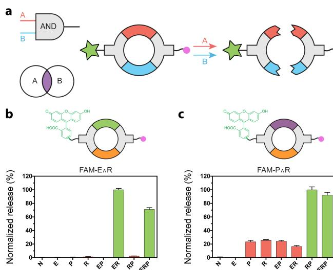
**Fig. 4** (a) Boolean AND-responsiveness is achieved through inclusion of two degradable moieties in parallel between gel (pink circle) and small molecule (green star). FAM is selectively released from gels for conditions involving (b) enzyme AND reductant, or (c) light AND reductant. X-axis labels indicating treatment conditions, release normalization criteria, histogram bar color, and error bar format match that described in Fig. 2.
