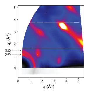
**Figure 5.** 2D scattering image obtained from GIWAXS of dry eADF4(C16) coatings on silicon wafer (24 hrs coating time) after conversion to  $(q_n, q_z)$  space, showing anisotropic scattering by the (200) planes of β-sheet crystallites along the  $q_z$  axis. Scattering arising from the eADF4(C16) coating occurs in the range of 0.8 Å<sup>-1</sup> < |q| < 1.8 Å<sup>-1</sup>, while scattering from the underlying silicon and native oxide layer is visible at |q| > 1.8 Å<sup>-1</sup>.
