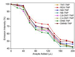
Fig. 3 Decrease in fluorescent intensities upon addition of various nitro analytes (1mM) followed by TNP (1mM) in aqueous medium.
