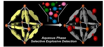
Scheme 1 Fluorescent MOF based sensor for highly selective nitro explosive detection in aqueous phase.
