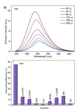
**Fig.1** a) Change in the fluorescence intensity of **1'** in water upon incremental addition of aqueous TNP solution 1 mM.  $(\lambda_{ex}=320, [1']=0.5 \text{ mg/mL})$ . b) Efficiency of fluorescence quenching obtained for different analytes
