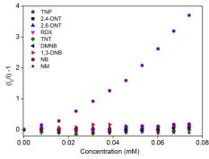
Fig. 2 Stern-Volmer (SV) plots for various nitro analytes in water. ([1'] = 0.5 mg/mL)
