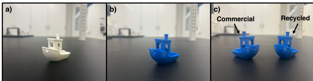
Fig. 7 3D printed 3DBenchys of 6.0 cm length, 3.1 cm width and 4.8 cm height from the (a) recycled white filament and (b) recycled blue filament. (c) Comparison of commercial and recycled filaments on a final 3D printed object.
