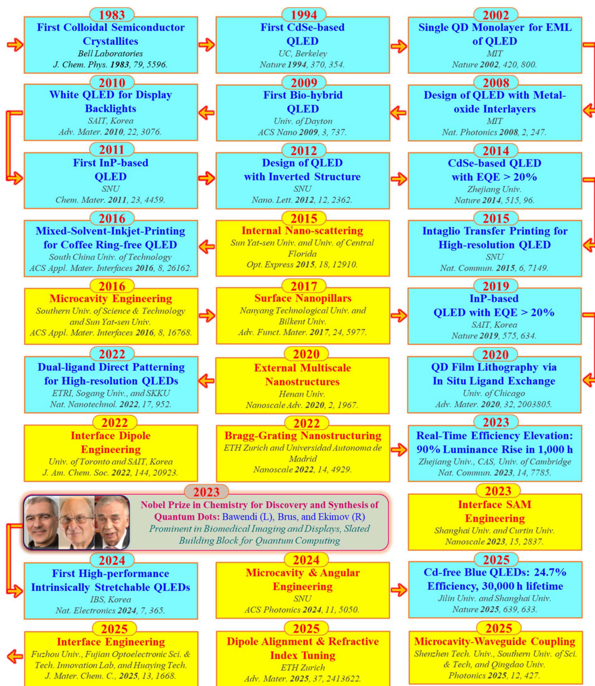
Fig. 1 Milestones in the evolution of QLEDs (cyan colour background) and advancements in LOC efficiency of QLEDs (yellow colour background).
